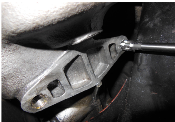
Tapping thread to fit coil. This side has been threaded and coil inserted. Tap has been marked at 20mm.
